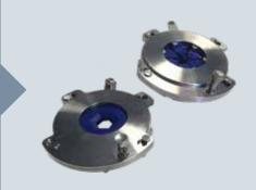
DJM developed uniquely constructed infinitely adjustable dosing irises for the production of cylindrical, oval and round shaped products. There are different iris-versions (DF50, DF70 and DF90) for maximum product diameters of 35, 55 and 75 mm respectively.
